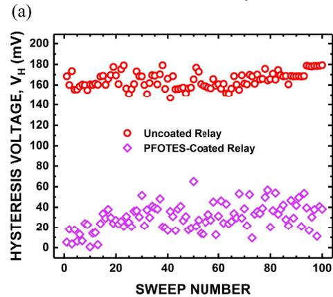
Fig. 9. (a) Measured  $I$ - $V$  characteristics. (b) Evolution of measured  $V_H$  for PFOTES-coated MEM relay operated over 100 gate voltage sweeps at  $V_{DS} = 1$  V and body-biased conditions. These data indicate significantly decreased value and variability in  $V_H$  due to the PFOTES coating.  $L = 8 \mu\text{m}$ .
