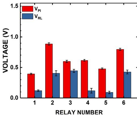
Fig. 6. Measured switching voltages for multiple relays operated at  $V_{DS} = 1$  V,  $V_B = -14.5$  V.  $L = 8 \mu\text{m}$ .
