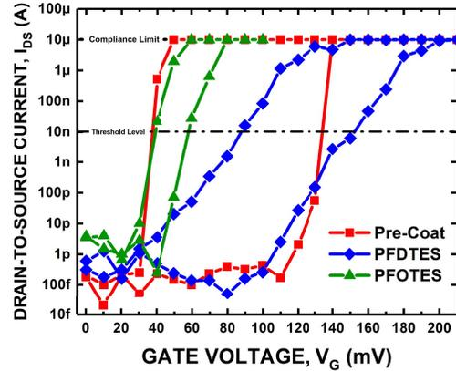
Fig. 8. Measured  $I$ - $V$  characteristics for body-biased relays, showing the effects of antistiction coatings.  $L = 12 \mu\text{m}$ .
