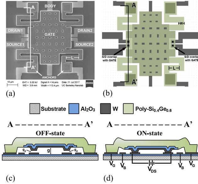
Fig. 1. Plan view (a) scanning electron micrograph and (b) mask layout of the six-terminal relay design used in this paper. The flexural beam length  $L$  and width  $W$  are indicated. The cross section A–A' is shown in (c) OFF-state and (d) ON-state. In the ON-state, surface adhesive force is introduced resulting in hysteresis.
