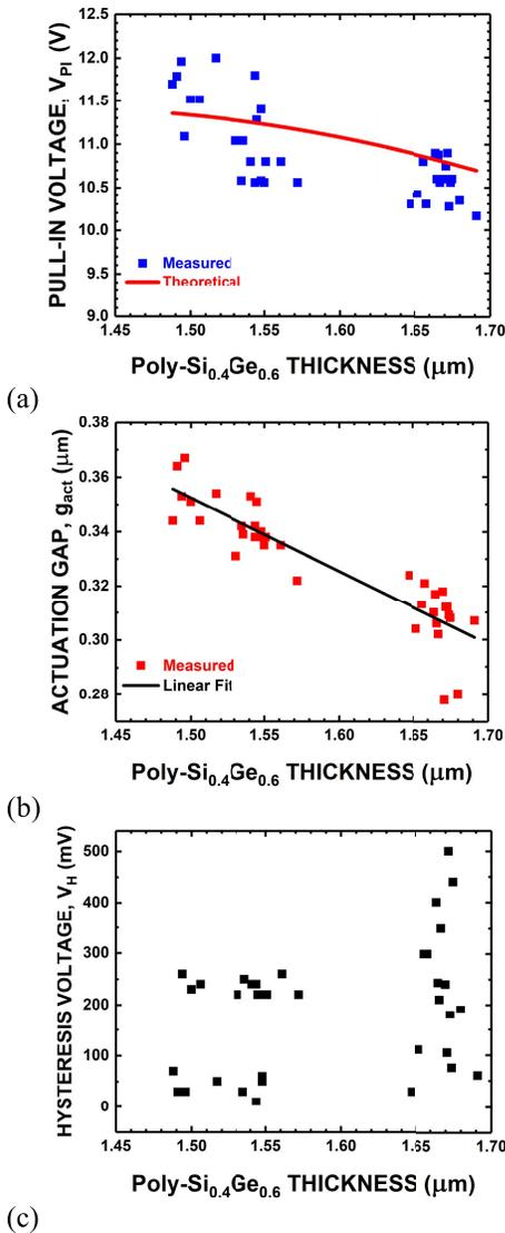
Fig. 5. Measured impact of process-induced variations in poly-Si<sub>0.4</sub>Ge<sub>0.6</sub> thickness on (a)  $V_{PI}$  for relay operated at  $V_B = 0$  V, (b) actuation gap  $g$ , and (c) hysteresis voltage  $V_H$ . The negative correlation between the structural layer thickness and actuation gap size is due to the reduced out-of-plane deflection for a stiffer structure.  $L = 12 \mu\text{m}$ .
