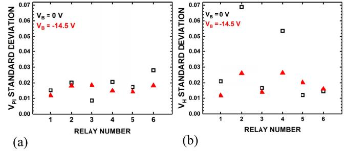
Fig. 4. Measured variability in (a)  $V_{PI}$  and (b)  $V_H$  for multiple relays operated at  $V_{DS} = 1$  V with  $V_B = 0$  V or  $V_B = -14.5$  V. Body biasing generally decreases variability in  $V_{PI}$  and  $V_H$ . The current compliance limit was set to  $10 \mu\text{A}$ .  $L = 8 \mu\text{m}$ .
