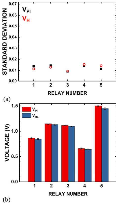
Fig. 10. Measured (a) variability in  $V_{PI}$  and  $V_H$  and (b) switching voltages for multiple PFOTES relays operated at  $V_{DS} = 1$  V and  $V_B = -16$  V.  $L = 8$   $\mu\text{m}$ .
