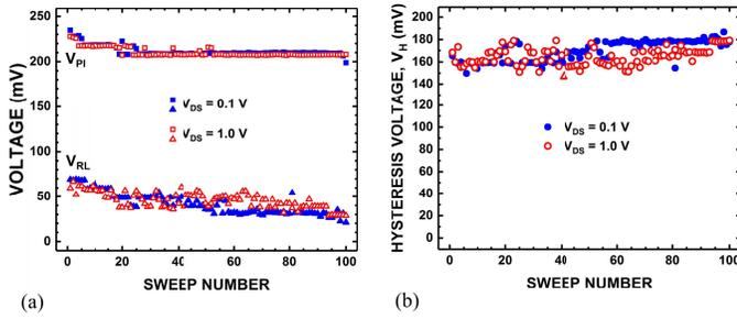
Fig. 3. Evolution of (a) relay switching voltages and (b)  $V_H$  for relay operated at  $V_B = -14.5$  V and various values of drain-to-source voltage  $V_{DS}$ . The current compliance limit was set to  $10 \mu\text{A}$ .  $L = 8 \mu\text{m}$ .
